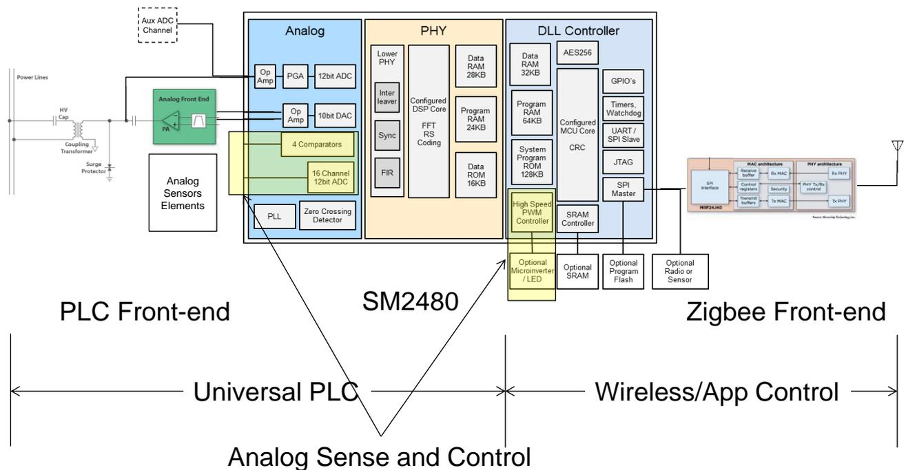
You can see that all the analogue sensing and analogue and digital outputs are built into the SM2480. There are also high accuracy Pulse Width Modulator outputs which is basically the inverter DC /DC and DC/AC inverter stages. The second 32-bit MCU runs all the software in the inverter, which includes the MPPT algorithm etc.
