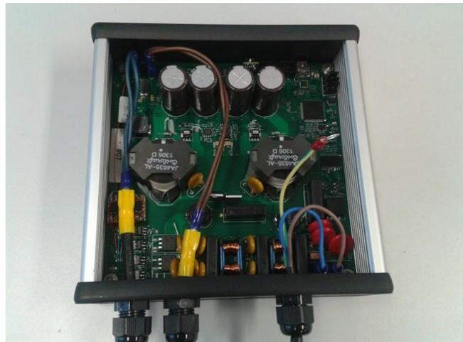
External and Internal View of the Evaluation Micro-Inverter
