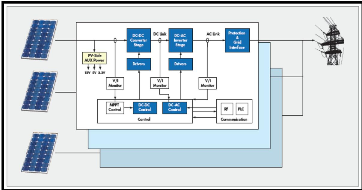
There are two basic signal paths: a “power path” where the DC voltage generated by the solar panel is converted to AC power and the “control and communication path”. The control function monitors the various voltages and currents in the “power path” and implements control loops to create and optimize the grid compatible AC power output. The communication function implements one or more of the grid-based standards discussed above to implement panel or overall inverter function monitoring.
